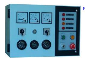
PowrWorld Standard Control Panel is the basic configuration for normal operation and usage, it is of some advantages such as easy to operate, various function and well protection. Operative buttons such as Turn On, Per-heat, Starting, Stop (Emergency Stop) on the panel. While malfunction occurs, control panel will stop the generator and also alarm with light or buzz.
